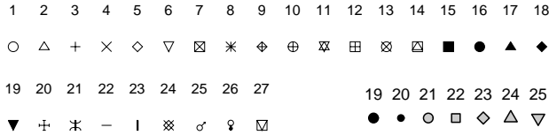
Figure 4.2: Plotting symbols or marks, specified by pch = n . Those on the left of the second row are only available on graphsheet devices, and those on the right of the second row only in R (where the fill colour for 21 to 25 has been taken as light grey).
