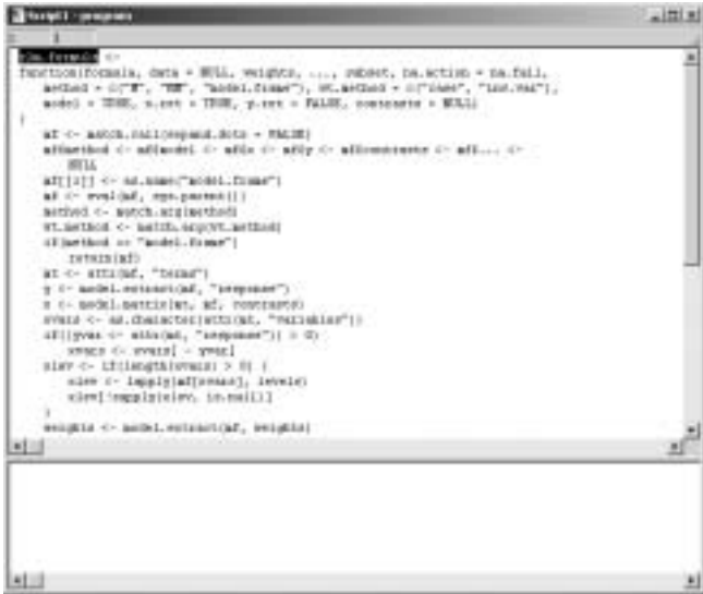
Figure B.2: A script subwindow. The definition of rmlm.default was inserted by highlighting the name (as shown), right-clicking and selecting Expand Inplace.
